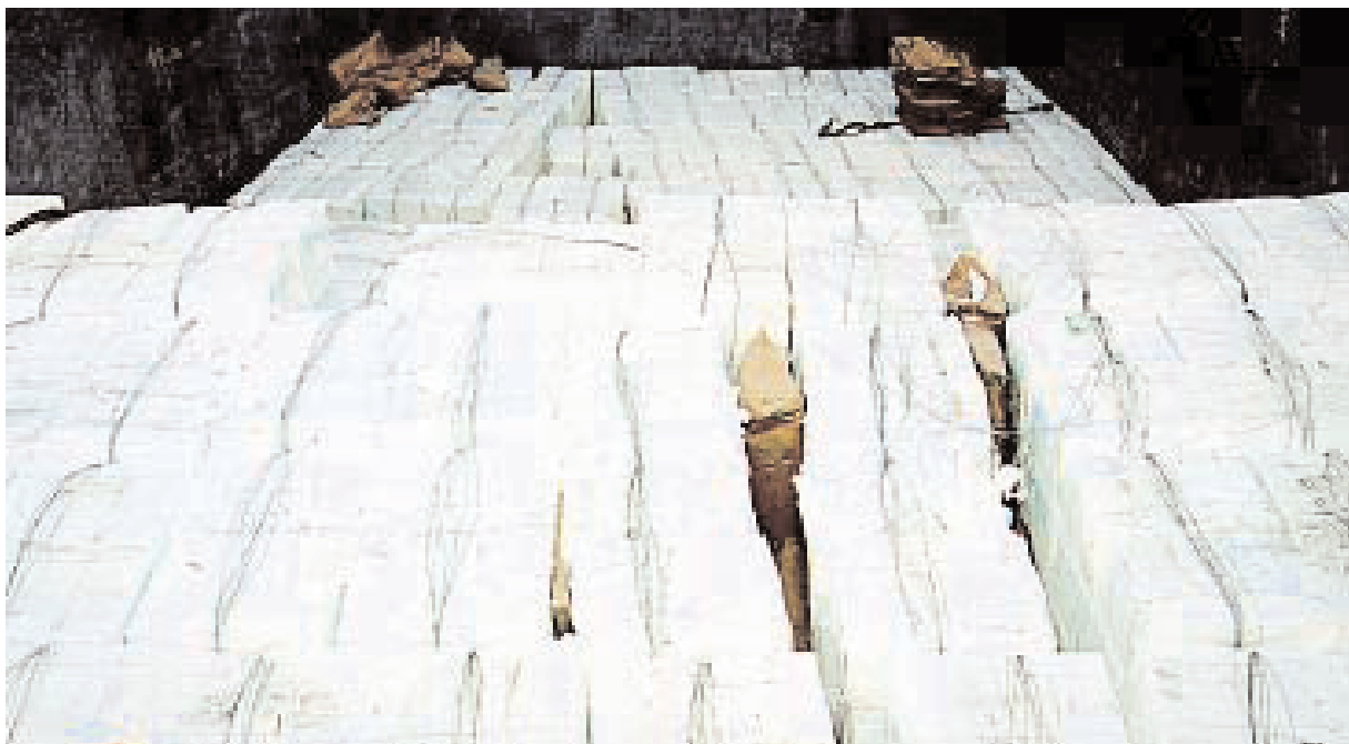
Unitised wood pulp. Note the use of airbags to secure the stow
