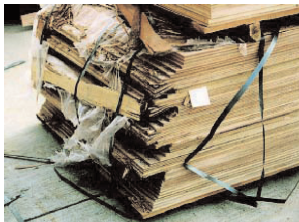
Plywood bundle showing torn plastic sheeting with loose and broken strapping bands'
