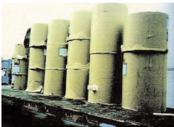
Reels of newsprint showing tears and cuts both in the wrappers and paper before shipment
