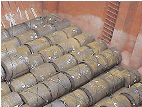
Photo 1. Coils of hot rolled steel These coils are usually between 1.20 and 4.50 metres in diameter and weigh between 5 and 15 tonnes each
