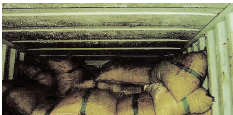
Condensation from the container roof has dripped on to the bags
