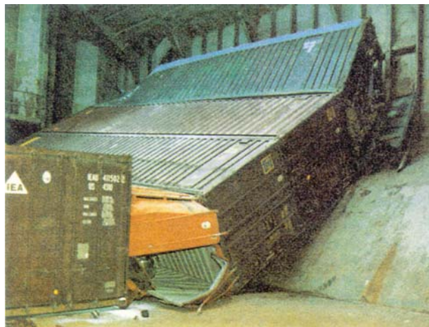
Collapse of stow: Nine containers were damaged in this incident. Note the damaged container at the base of the stow
