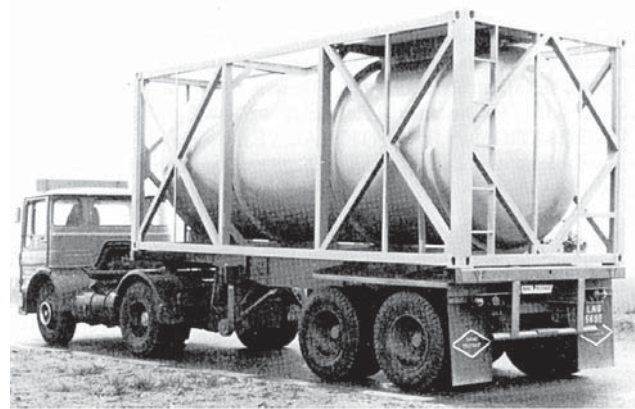
20ft x 8ft tank container. May contain highly corrosive and/or toxic liquids. Courtesy Jane's Freight Containers
