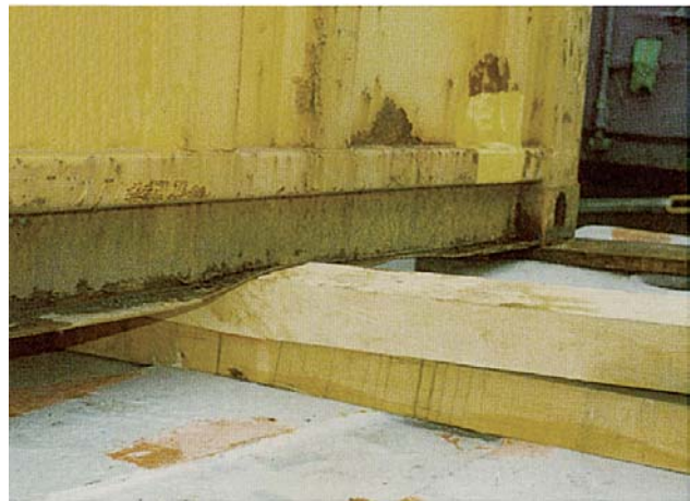
When stowed like this skirts and bottom rails collapse and general slackness develops in the stow
