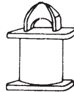
5. A 6" spacer with single stacking cone, sometimes supplied with two opposing cones. Used to bring the tops of unequal size adjacent containers in stack to the same horizontal line so that screw-bridge fittings may be attached to corner castings (see 7.)
