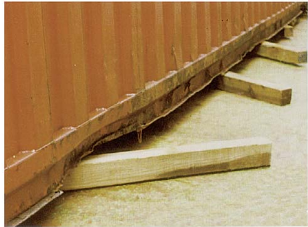
NEVER stow ISO containers on their bottom rails or skirts. ALWAYS stow ISO containers on their corner castings only
