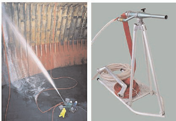
Typical hold cleaning equipment: crew operating a Toby gun and a Toby gun from Stromme
