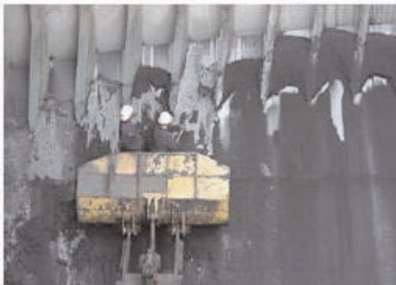
Shore bulldozer/cocoa beans and shore personnel cleaning holds.
