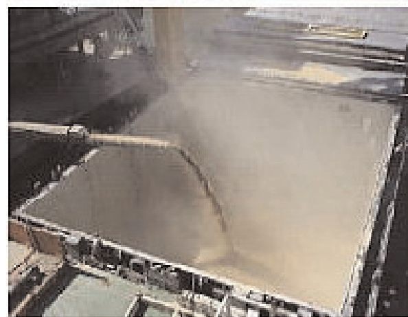
Grain dust cloud presents a health hazard. Loading barley (bottom)
