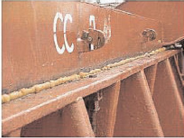
Do not use foam to seal hatches
