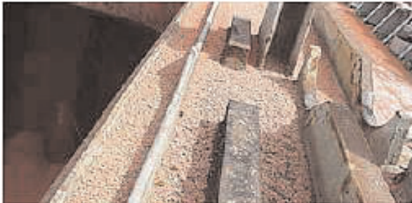
Coaming/trackway covered in fertiliser
