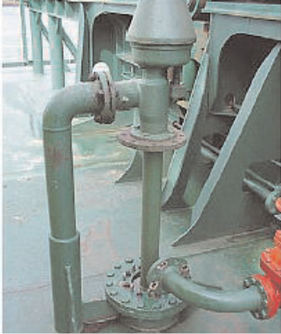
Hold cleaning equipment in the stowed position above the deck. Note the flange on the deck wash line
