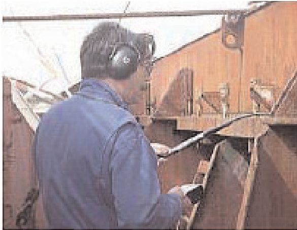
Ultrasonic hatch testing for leaks
