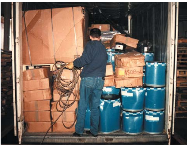
Photo 1: Poorly stuffed container – note the damaged packages, the pallet on top of cartons and the apparent lack of securing arrangements
