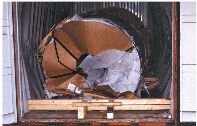
Photo 3. Note the damage caused to the container by the poorly secured coils
