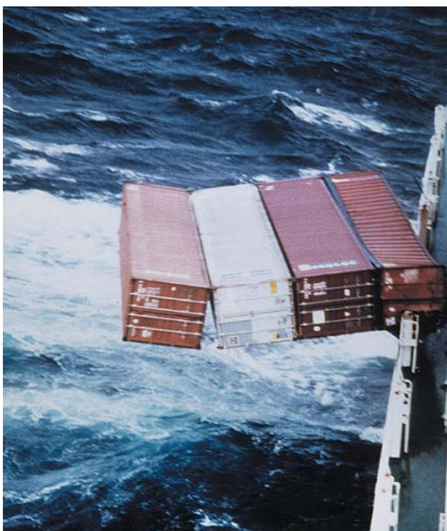
Photo 5: The ultimate lashing failure
