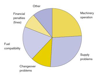
Nine ships reported having problems with machinery operation when operating on low sulphur fuel, which included fuel oil lubrication of pumps and nozzles, sticking fuel pumps, generator starting problems, fuel oil leakages and delayed pick up speed of engines.
