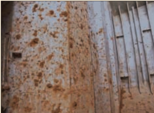
▲ 1. Warning signs: such heavy splattering on the hold bulkhead during loading is an indication that at least some of the cargo has experienced 'flow state' due to impact.
