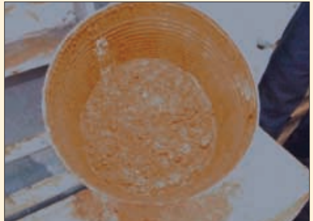
▲ 3. Showing the same sample but after 25 strikes of the can on a hard metal surface. Note the flat surface and free moisture visible in the surface layer, indicating that the sample has liquefied.
