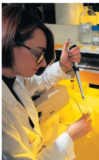
A solution of silver nitrate in distilled water is regularly used as a simple test for the detection of seawater contamination of ships' cargoes. Whilst the test is a useful preliminary test for saline contamination it should be considered as indicative only. It has limitations and should not be relied on as definitive proof of saltwater contamination; more detailed laboratory analysis will be required to confirm this. The reaction is shown below:
