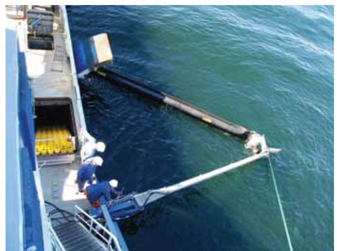
▲ Figure 32: An in-built single ship recovery system. Boom stored in a compartment at the side of the vessel is deployed through an opening by an on-board crane. The opening also allows entrained oil to be recovered by the in-board skimmer, here comprising six sets of brushes in a conveyor arrangement (Image courtesy Lamor).
