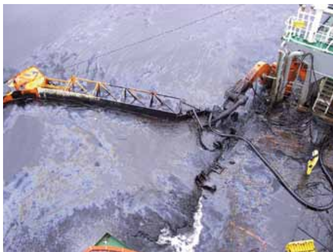
▲ Figure 33: Rigid sweeping arm attached via hydraulic crane to the recovery vessel. The low freeboard and large swell encountered made conditions on deck hazardous for the vessel crew (Image courtesy WSA Cuxhaven).
