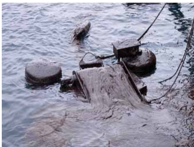
▲ Figure 16: A belt adaptor added to enhance the capability of the base weir skimmer in highly emulsified fuel oil. The high viscosity of the oil prevented its flow towards and over the lip of the weir. Instead, the toothed belt adaptor 'grabbed' the oil enhancing the efficiency, with the cohesive energy of the oil causing the remaining oil to 'flow' toward the skimmer (Image courtesy Ro-Clean Desmi/Danish Navy).
