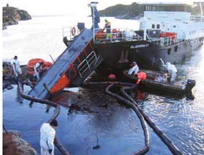
▲ Figure 15: A belt skimmer on a large recovery vessel. The belt, constructed from a mesh, allows water to drain through and encourages adhesion of the oil. The oil is lifted on-board and is scraped off to storage.
