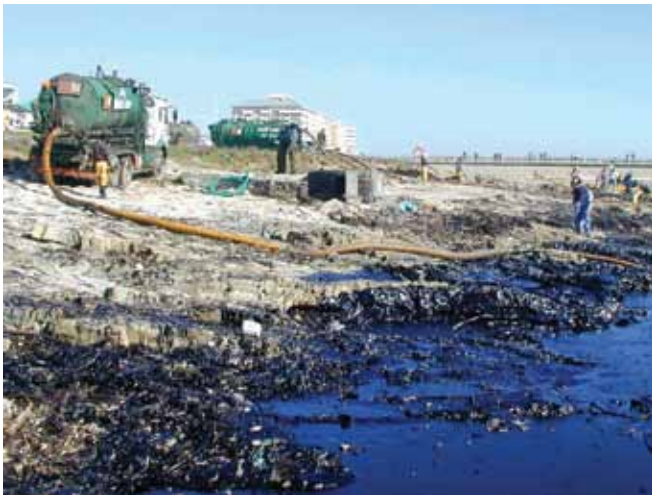
▲ Figure 8: The widespread availability of vacuum systems make these devices ideally suited to recovery of oil on or near the shoreline.
