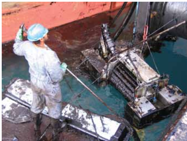
▲ Figure 17: Mechanical drum skimmer deployed in a port area. Teeth on the rotating drum draw the oil towards the device where it is recovered into the drum and pumped to storage. The drum is constructed from a mesh to minimise recovery of water.
