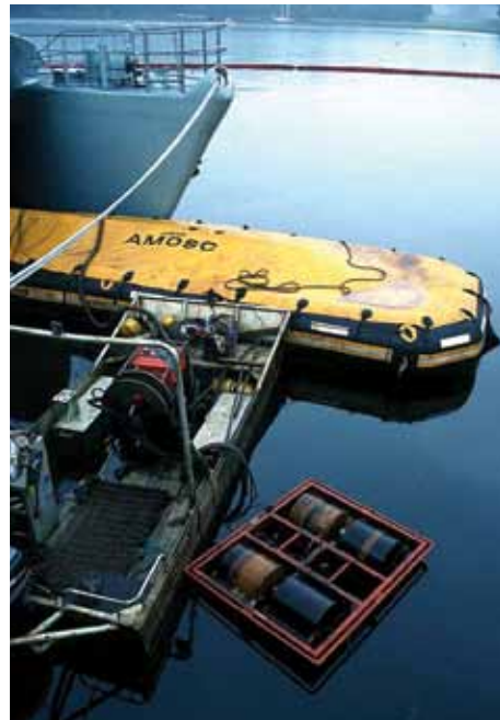
◀ Figure 26: A drum skimmer recovering oil to an inflatable storage barge.
