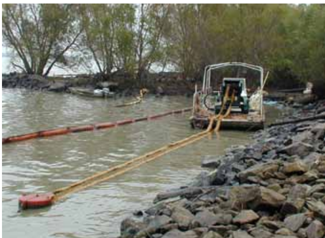
▲ ▶ Figures 6 and 7: Horizontal and vertical oleophilic rope skimmers. Interwoven sorbent loops form a continuous mop which floats on the surface to which the oil adheres. The mop is pulled back to a roller and the oil squeezed to a storage tank. Rope mop skimmers are useful to recover oil from among debris, ice and other obstructions.
