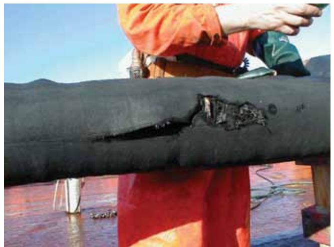
▲ Figure 23: Burst hose as a result of excessive internal pressure from pumping highly viscous oil (Image courtesy NOFO).
