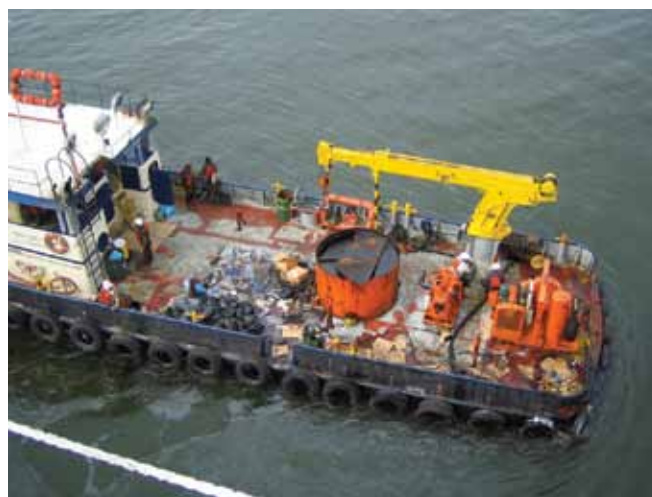
▲ Figure 24: A workboat with limited recovered oil storage on deck.
