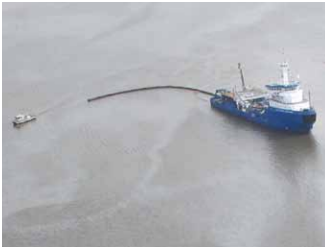
▲ Figure 29: Boom towed in a U configuration with a skimmer deployed from the main recovery vessel.
