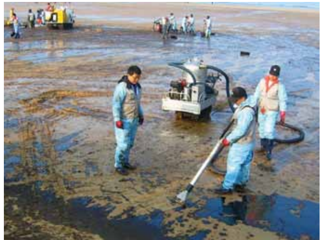
▲ Figure 9: Portable vacuum systems can facilitate the recovery of oil on sand beaches and rocky shorelines. The compact system allows work in areas that are otherwise difficult to reach, although storage is limited.
