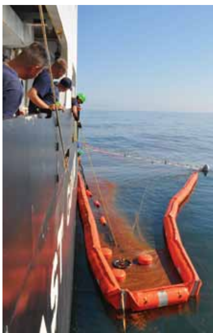
◀ Figure 31: A single ship recovery system comprising inflatable boom attached to an outrigger and a high capacity free-floating weir skimmer mounted on a Coastguard vessel. The high freeboard allows deployment on the leeward side in calmer waters (Image courtesy USCG).
