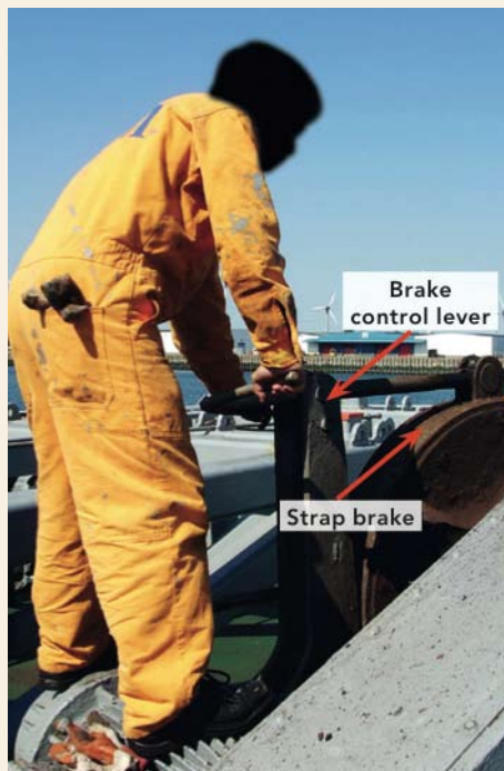
Simulation of A/B attempting to secure the brake as the chain ran out
