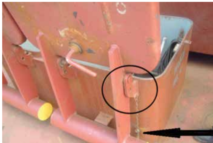
Ship's crew should ensure that the locking pins are always properly secured whenever the booby hatch is in the open position
