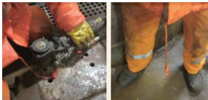
Dangling lanyards pose a potential snagging hazard
