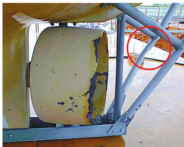
Loss of bow fendering and damage to the 'overall spray system' are both caused by entry into the water and cracks in the GRP fabric of the craft by the same means. Damage to stern assemblies, rudder nozzles and bilge grab rails is mainly caused by launch and
