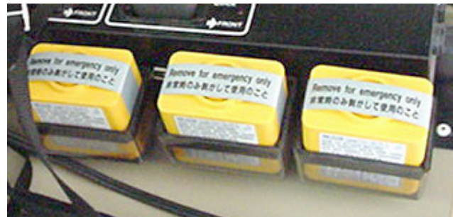
Emergency power source
