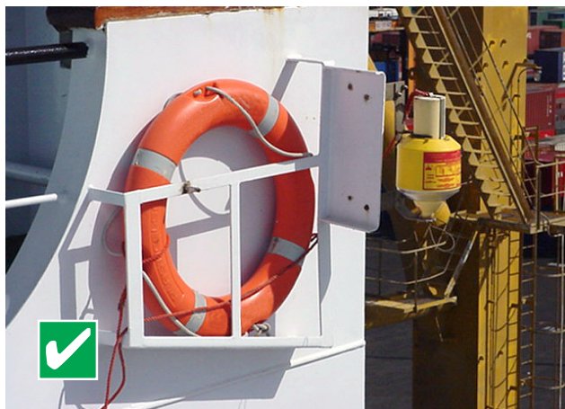
Lifebuoy and smoke float correctly rigged
