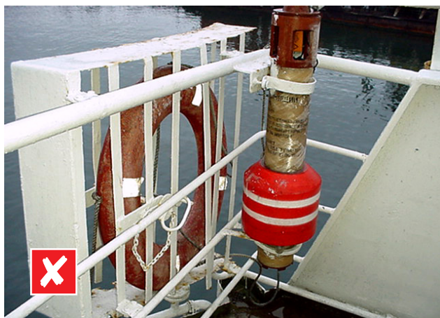
Smoke float wrongly rigged inboard of bridge wing
