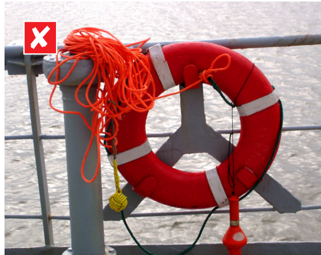
Wrong: Lifebuoy rigged with line at pilot boarding
