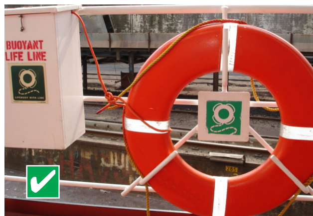
Correct: Lifebuoy with line
