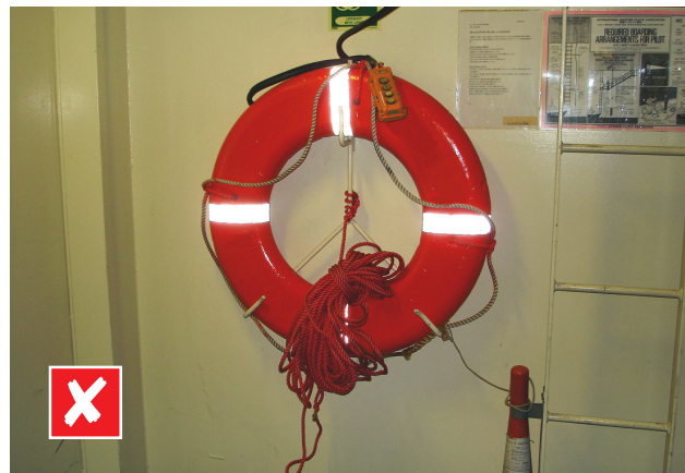
Wrong: Lifebuoy rigged with light & line
