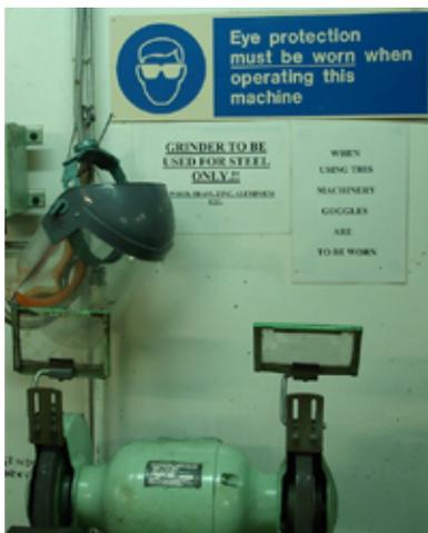
Engine room workshops are usually fitted with pedestal and bench grinders. UK Club ship inspectors sometimes find grinders on board with no safety guard fitted. These are sometimes removed, or not used, by crew who do not fully appreciate the risk of grinding disks shattering. A properly fitted guard will shield the user from shards of grinder disk in the event that the disk shatters while in use.
