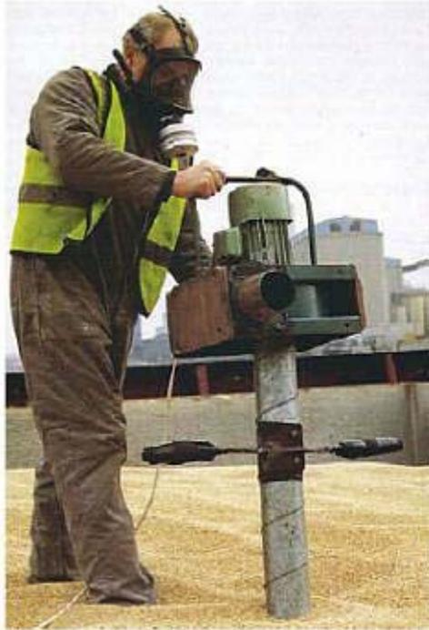
*Ventilating the cargo prior to discharge.*
