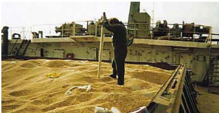
*Probing aluminium phosphide in retrievable sleeves into a bulk cargo*
