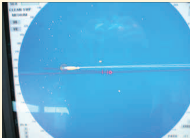
▲ 2. Radar picture showing correct positional information
