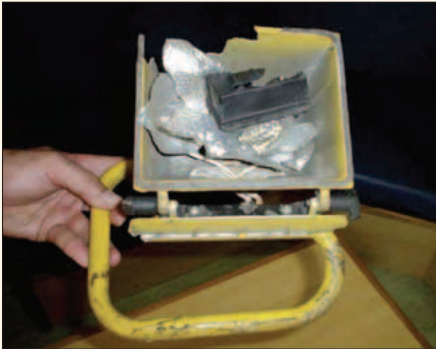
▲ Figure 2: remains of the non-intrinsically safe halogen lamp that caused the explosion
