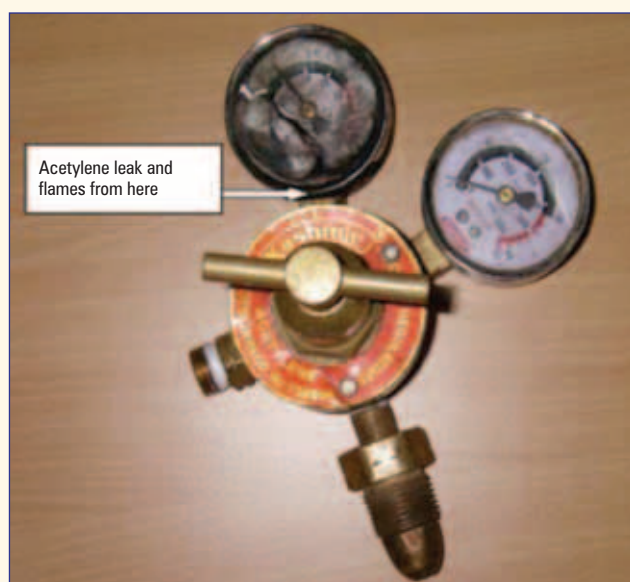
▲ Figure 3: Wrongly fitted acetylene regulator pressure gauge
