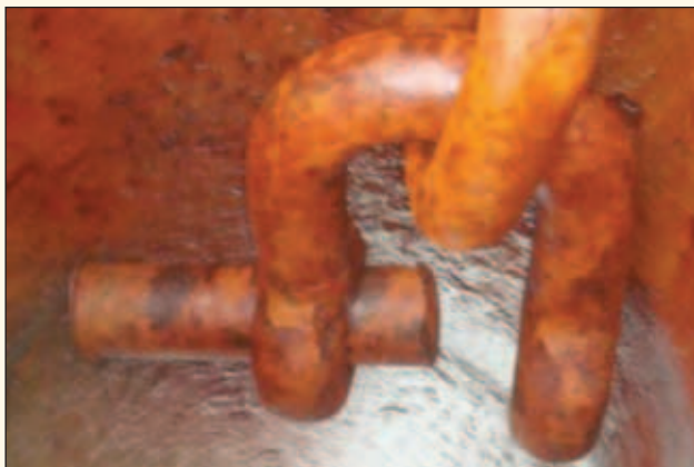
▲ Figure 1: 'D' shackle showing main pin displaced and anchor missing
