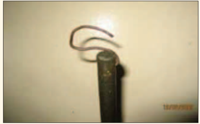
▲ Figure 3: View of open wire tail fitted on handle's free end for hanging spanner
