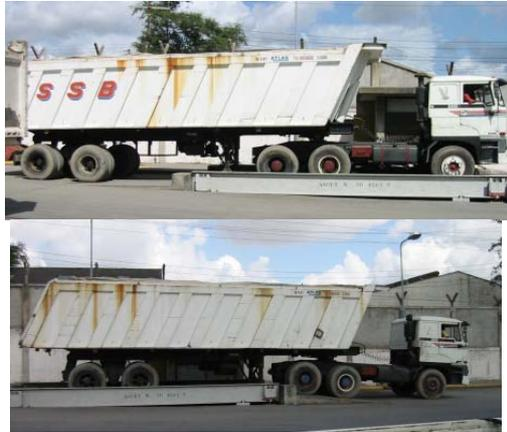
We are advised that instead of uncoupling the trailer the front end of the unit is weighed, the unit then drives through leaving the rear axle on and another reading taken. The readings are then added together. This is done both empty and full the difference being the weight of the commodity.
