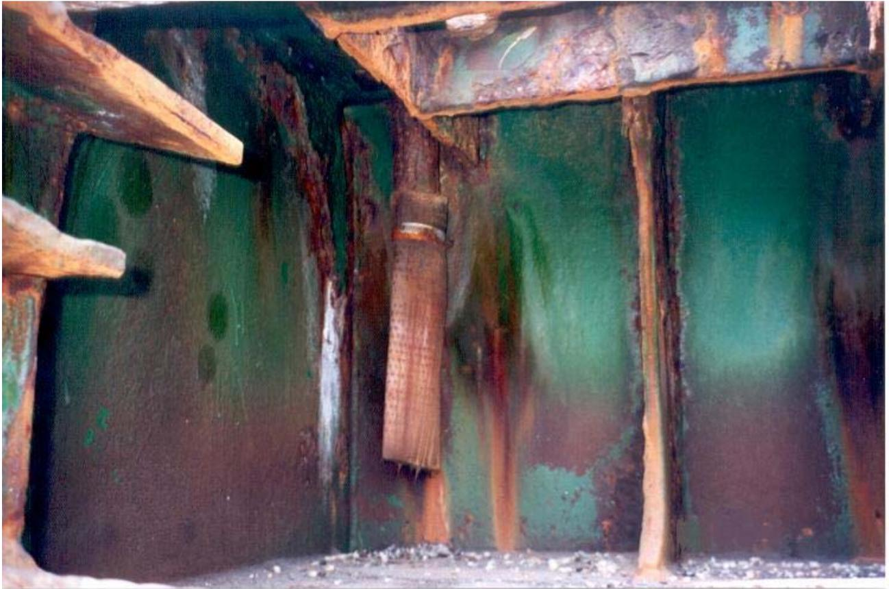
It is essential therefore, that whatever approved device is fitted at the drains, it is in position and fully operational at the commencement of the voyage. Water ingress arising from wasted or missing sections of non return ball valve arrangements, open pipes, or even hardened lengths of canvas hose, cannot usually be defended as damages arising from heavy weather.
