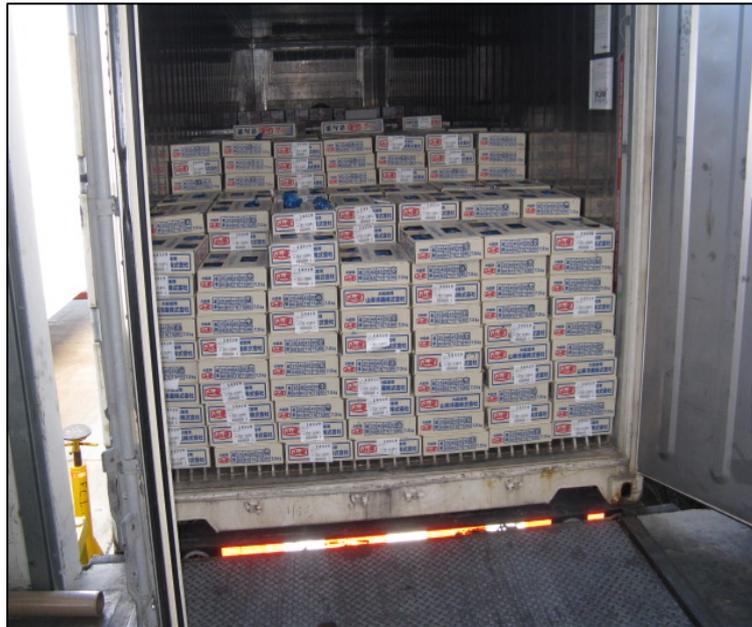
The terminal personnel should document, in part, the refrigerated container number, the temperature and vent setting, the weight of the container, cargo and chassis and the seal number on the equipment interchange receipt ("EIR").
