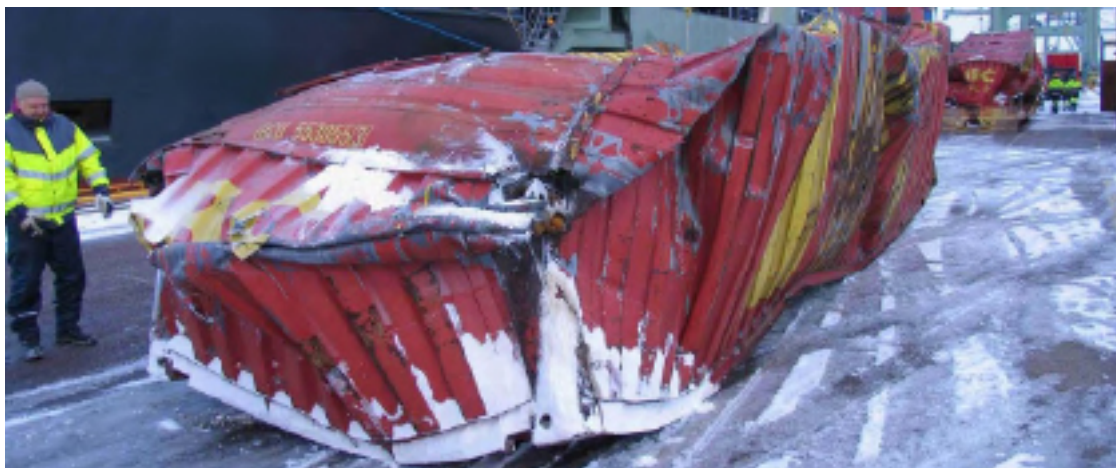
Image: the container discharged from the bottom of a collapsed stack
