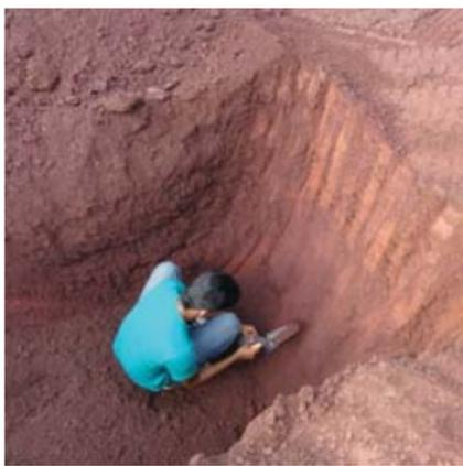
Ideally the stockpile should be flattened such that all parts of the pile are accessible and can be sampled. An excavator should be employed to cut slots into the sides of the pile, and to dig pits into the top to access the core of the stockpile. If an excavator is totally unavailable, this should be reported to your principal so that an amended sampling method can be agreed.
