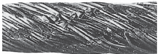
Abraded wire rope, showing localised damage to individual wires
