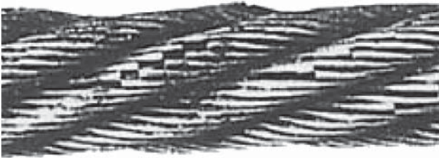
Fatigue-induced wire breaks are characterised by flat ends on the broken wires
