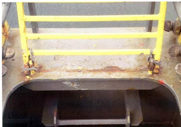
rung that would ordinarily had secured it to the pad eyes located on either side of the lashing catwalk opening. The grating showed signs of rust and wear and tear and should have been identified by the vessel's crew as an item in need of repair during regular vessel inspections.
