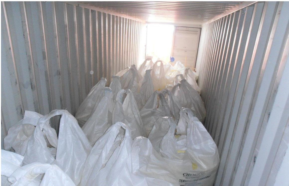
During transshipment operations in Hamburg one container in a large booking of bagged Sulphur (UN4.1, IMO 1350) being shipped from St. Petersburg, Russia to Qingdao, China suffered an accident. The following investigation found that the dangerous goods were not packaged and secured as per the regulations as described within the IMDG code. As a precaution other containers in the same booking were inspected. All were found to be inadequately packed and secured.
