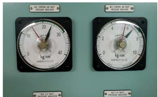
**Good start air pressure with safe operational limits marked**
