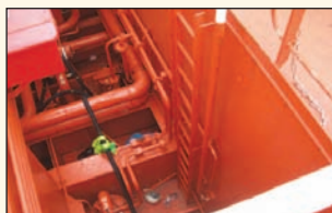
▲ Figure 2: Another view of deck area around Butterworth hatch showing the enclosed nature of the v space and possibility of heavy vapours settling at the bottom
