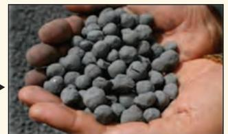
▶ Figure 2: DRI (B), Lumps, pellets, cold moulded briquettes
