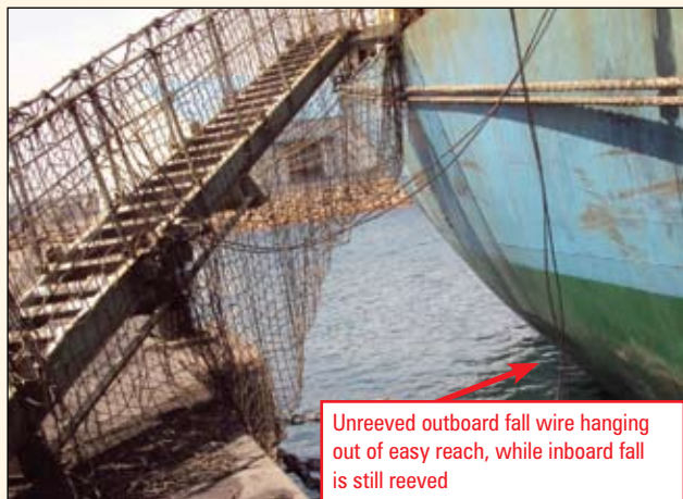
▲ Ship's accommodation ladder slewed outboard by a large angle and landed on the shore due to broad fendering on the berth and outboard fall wire temporarily unreeved from the side sheave
