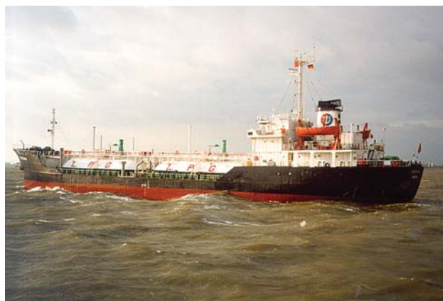
Pressurised LPG carrier with cylindrical tanks
