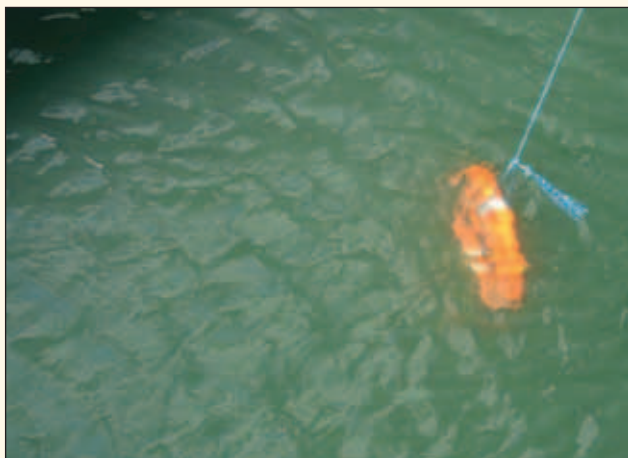
▲ Figure 2: Water-logged lifebuoy has insufficient buoyancy to float by itself
