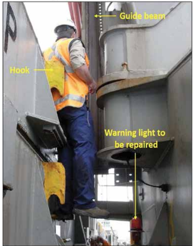
Likely position of the assistant electrician.
