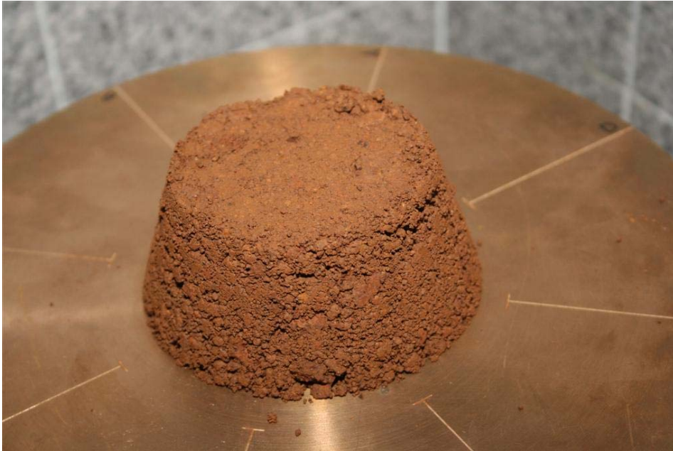
Image 1 - Typical shape of sample cone prior to testing
