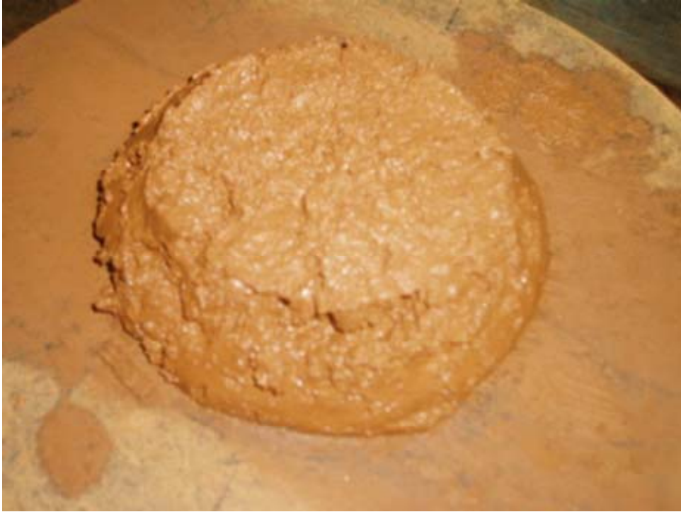
Image 3 - Sample cone after testing with 20mm expansion at base
