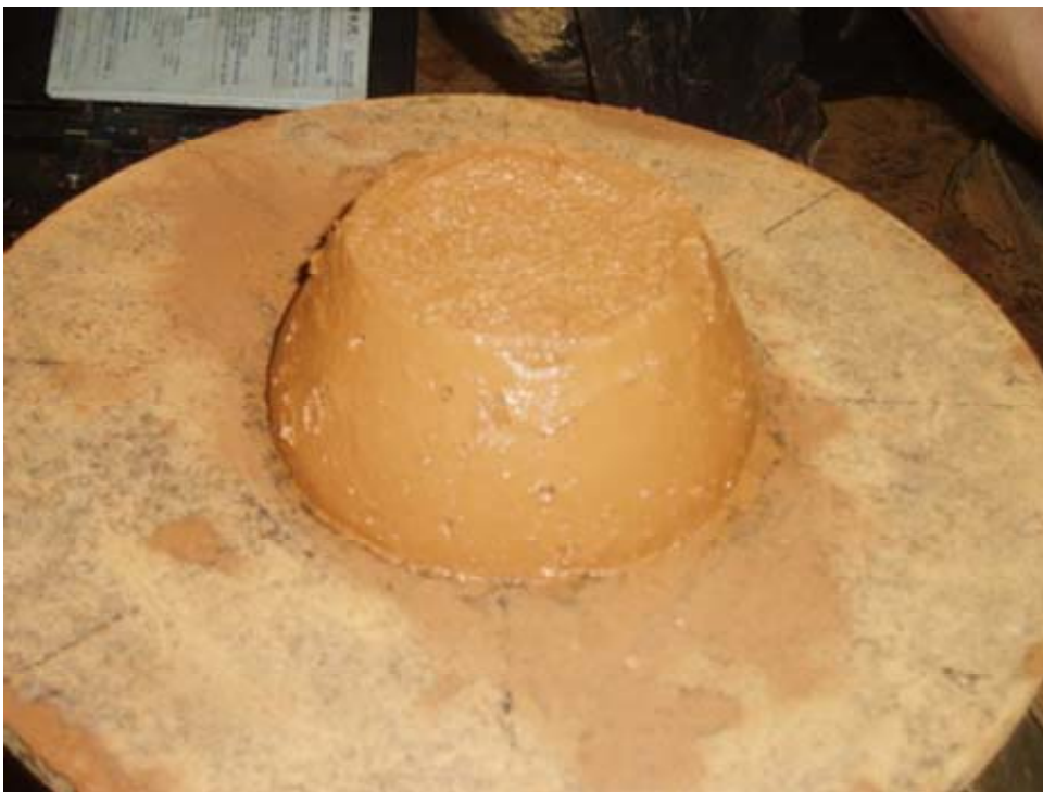
Image 2 - Change in shape of sample cone after testing, corresponding to a 6.5mm cone expansion
