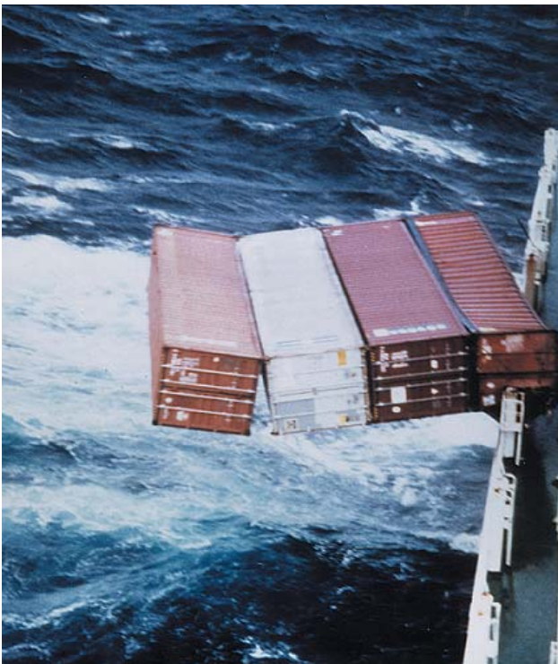
Photo 5: The ultimate lashing failure
