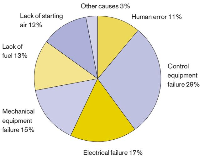
As is illustrated in diagram 5, control equipment failure accounted for the greatest proportion of main engine manoeuvring failures, this being mainly caused by the lack of or leakage of control air, along with other malfunctions. Blackouts (as discussed previously) accounted for the next highest cause of electrical failure. Of the 15% of mechanical failures, these were attributed to defects with pneumatic valves, start air valves and defects in reversing systems.
