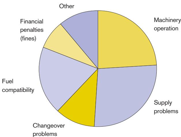
Nine ships reported having problems with machinery operation when operating on low sulphur fuel, which included fuel oil lubrication of pumps and nozzles, sticking fuel pumps, generator starting problems, fuel oil leakages and delayed pick up speed of engines.
