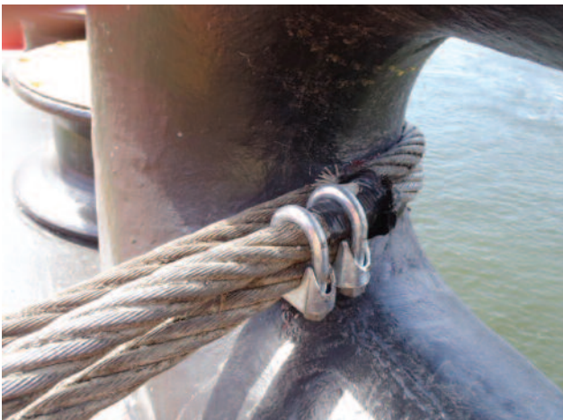
Correct way around but insufficient number of grips, too close together and wire tail too short
