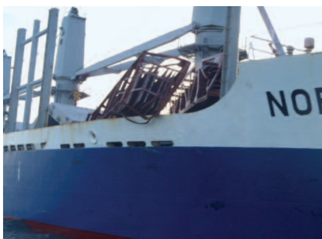
Damage to project cargoes
