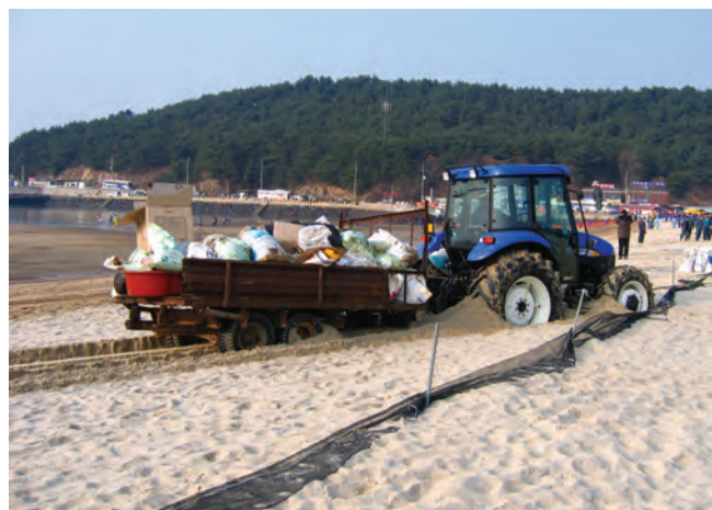
▲ Figure 39: Loaded vehicles can sink into soft substrates. This may cause additional damage and oil to become mixed with otherwise clean sediment.
