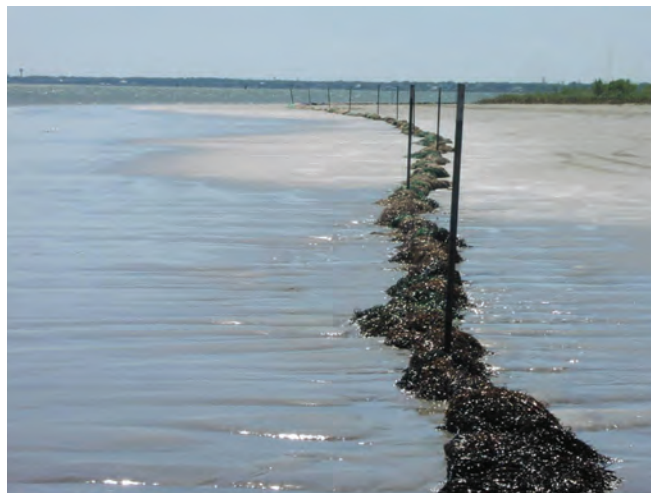
▲ Figure 7: Snare strung across an estuary to catch floating oil. The open structure and large surface area of the material are particularly suited to the recovery of viscous oils.
