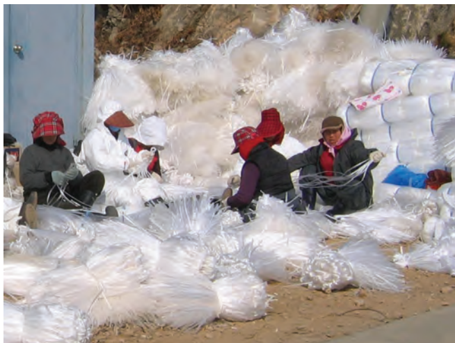
▲ Figure 6: Local villagers constructing snares from strips of polypropylene. The manufacture of sorbent from locally available materials can be cost effective in terms of price as well as efficiency of transport.
