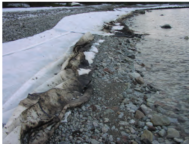
▲ Figure 5: Continuous flat sorbents, such as this sheet laid on a shoreline, are characterised by a high surface area to volume ratio. The large scale use of sorbent in this manner should be balanced against the generation of considerable volumes of potentially unsoiled waste.
