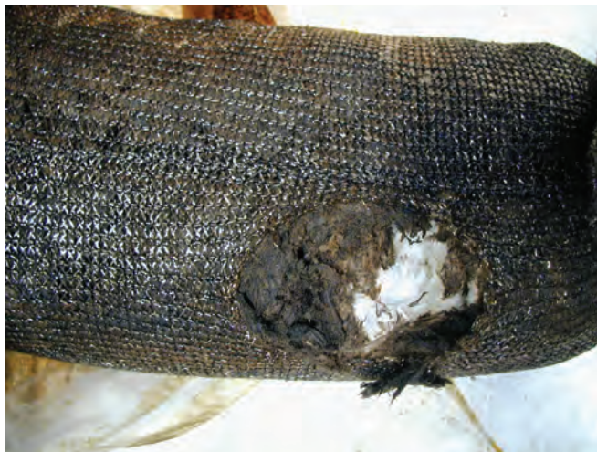
▲ Figure 4: The surface of a continuous, homogeneous sorbent boom cut away to show only partial use. The inner volume remains unsoiled, either because the boom has been deployed for an insufficient period or because the oil is too viscous to penetrate into the structure.
