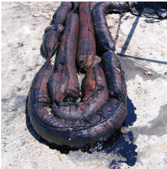
▲ Figure 14: Oil leaching from a recovered sorbent boom is a source of secondary contamination.
