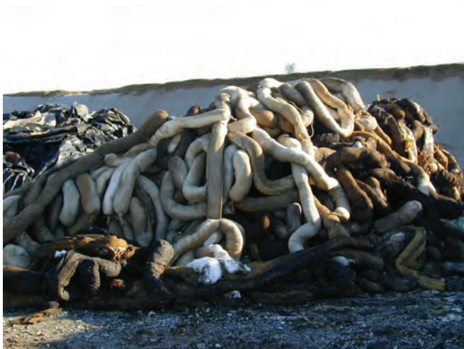
▲ Figure 15: Used sorbent piled in a temporary storage site. Compression will cause recovered oil to be squeezed from the boom and care is needed to avoid secondary contamination.
