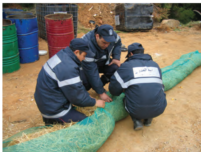
▲ Figure 2: Improved sorbent booms constructed from straw and netting. Such booms are cheap and easy to construct and can provide effective short-term protection when deployed in suitable areas.
