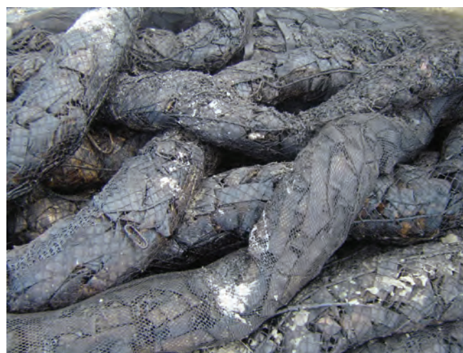
▲ Figure 3: Strips of polypropylene enclosed in netting. The loose inhomogeneous structure of the boom may allow oil to readily penetrate into the structure allowing inner surfaces to adsorb oil but the enclosing netting may be easily damaged.
