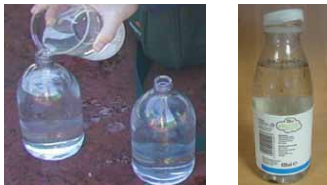
▲ Figure 12: Clear, narrow-mouth bottles (left) or plastic bottles (right) are not ideal containers for monitoring purposes.
