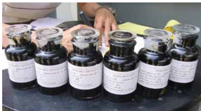
▲ Figure 11: Well labelled bunker samples in wide mouth glass jars (in this case split samples from a single tank).
