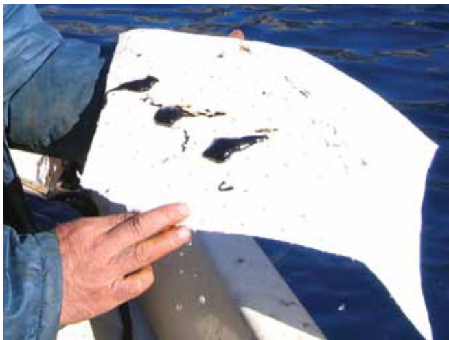
▲ Figure 6: Capturing floating oil with a clean sorbent pad.
