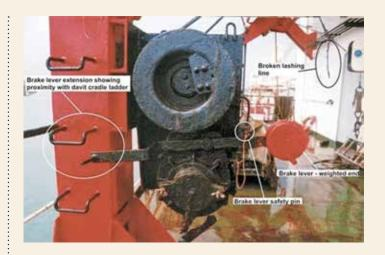
extended such that the handle was near the vessel's side to enable the person who controlled the brake, by pushing down, to view the lowering of the lifeboat. The handle was in very close proximity to the second rung of the aft cradle ladder (6 cm below and 5 cm away, see photo above).
