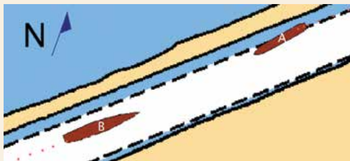
As the vessels close, vessel A experiences bank suction
