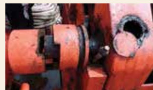
Windlass after accident
