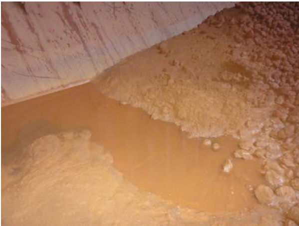
Water accumulation around the peripheries of bauxite stows.
