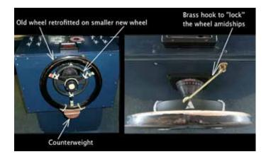
■ Editor's note: It never ceases to amaze how bad ergonomic design seems to be endemic in the maritime industry, as shown by the small wheel and inadequate helm position indication in this case. Additionally, the solutions brought to bear after the accident, although well meaning and probably effective, are a wellspring of improvisation and ironic adaptations. Would the airline industry allow such bad design or for that matter, such 'handyman' fixes?
