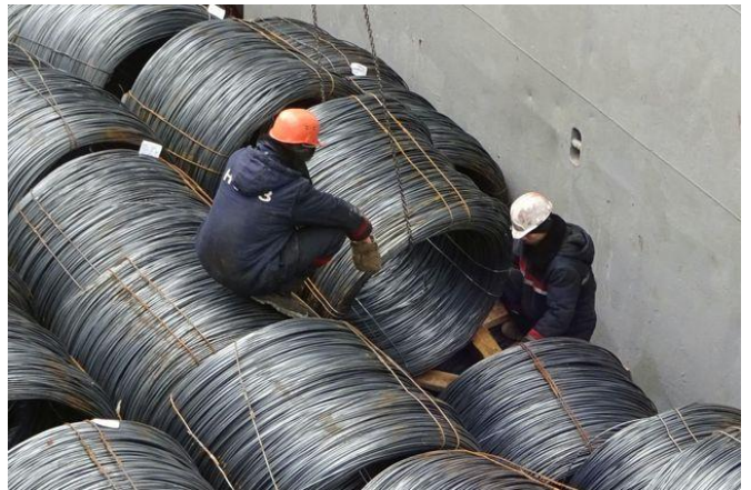
Coils of wire rod correctly stowed, timber dunnage applied to re-stow the collapsed coil
