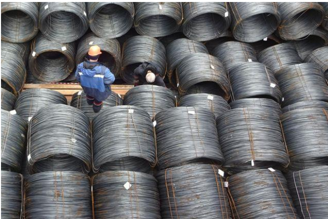
Coils of wire rod correctly stowed, timber dunnage applied to re-stow the collapsed coil
