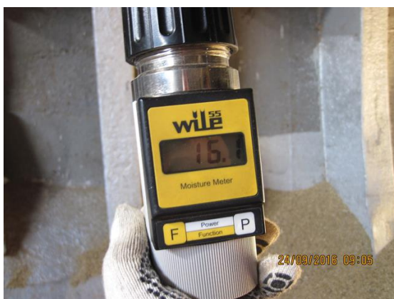
Portable moisture meter showing excessive moisture content
